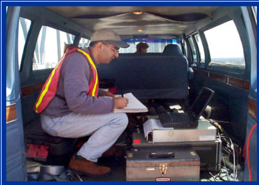
Data Acq. During Damper Testing
